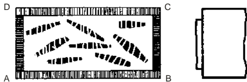
Fig. 7.3 : Rock Faced Stone Surface
